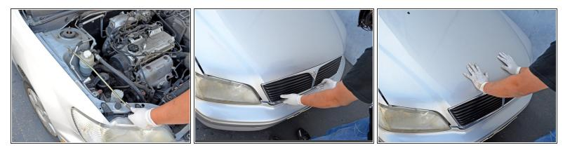
• Support the hood with one hand and use your other hand to place the hood prop rod back into its holder.
