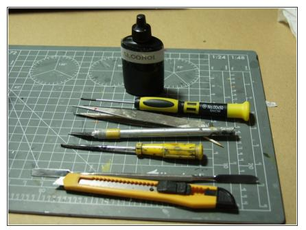
Here are the tools I used. You probably only need one knife. The alcohol is for removing adhesive residue and dirt.
