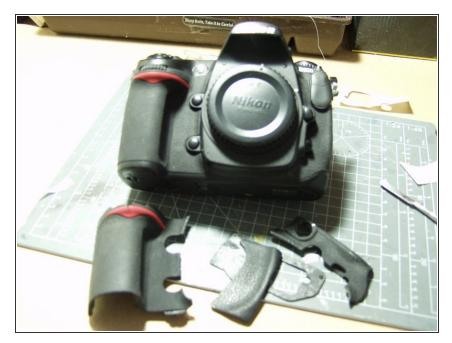
The finished job. Dust etc. should be removed from the new rubber with adhesive tape. Ensure everything is properly seated, and you're ready to go.
