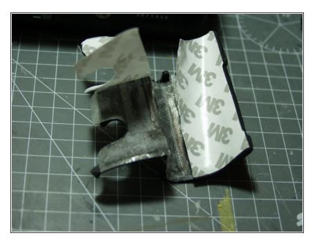
Take the new handgrip rubber and use tweezers to peel off the paper backing. These parts are very well cast, but the adhesive backing does not seem to be factory standard.
