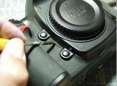
Clean off any adhesive left behind, and attach the new part starting by inserting the plastic tab back where the old one went and re-securing the screw. Carefully reattach the grip, tucking it in to the apertures in the body using the sculpting tool, or worn screwdriver - avoid piercing the rubber.
