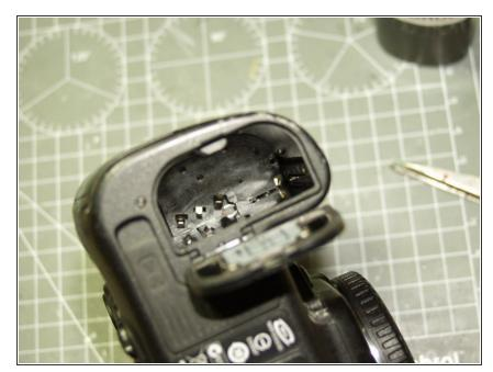
• The grip is attached to the body via a tab which is fastened by a small screw, that is accessible from the battery compartment. Remove the battery, you can see it in the photo upper right towards the front of the camera. unscrew this and keep the screw safe.
