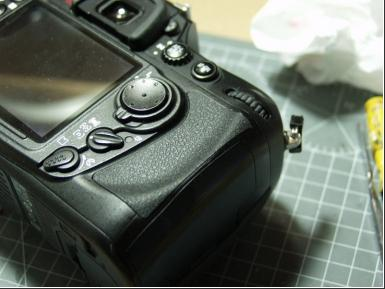
Remove the thumb grip. Note that here the old adhesive has melted, which required cleaning up with alcohol. The new rubber is easy to replace.
