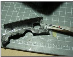
Remove the left hand grip, after turning the socket covers back out of the way. Remove dirt and adhesive residue. Cut the adhesive away from the socket hole before attaching. The rubber must be seated into the various body apertures, esp. behind the focus selection lever and beside the remote socket.
