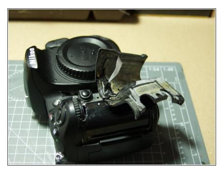
Getting the old grips off is easy using the sculpting tool, but note the right hand grip is secured with a screw, arrowed. See next step.
