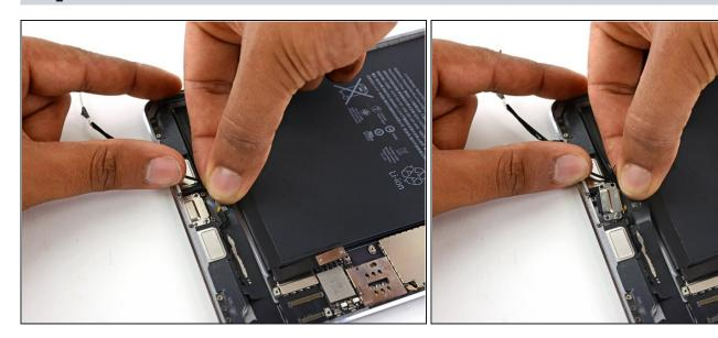
Begin to gently lift the Lightning connector cable up.
