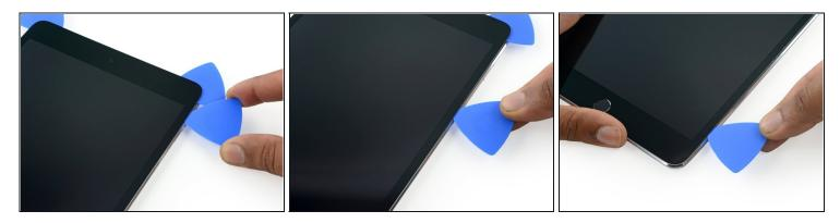
• Continue sliding the opening pick down the right edge of the iPad, reheating the edge using an iOpener if necessary.
