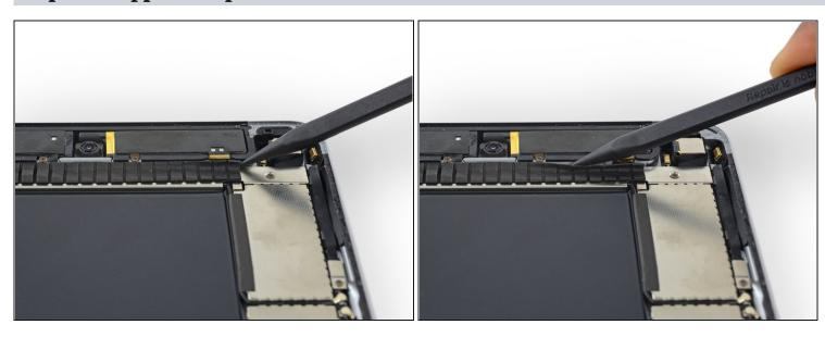
• Run the pointed end of a spudger between the looped tape and the plastic cellular antenna housing to make it easier to peel the tape up.
