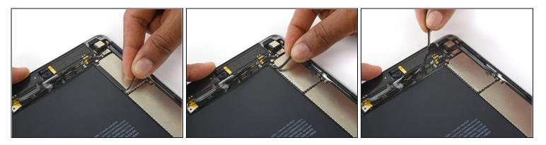
• Peel the upper antenna interconnect cable up off the logic board.
