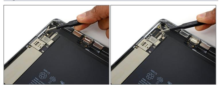
• Peel the lower antenna interconnect cables away from the corner of the rear case.
