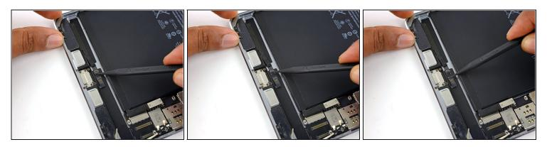
• Use the tip of a spudger to lift each of the two ZIF connector retaining flaps.
