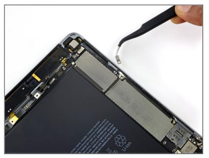
• Remove the volume control cable bracket.
