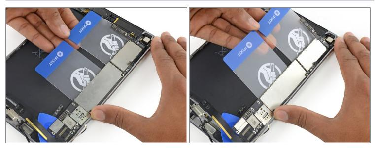
• Lift up on the edges of both plastic cards to pry the logic board from the rear case.
