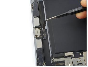
Remove any tape covering the ZIF connectors near the Lightning connector port.
