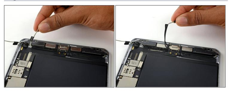
• Peel the left antenna interconnect cable up off the Lightning port cable.
