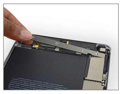
• Remove the upper component cable bracket.
