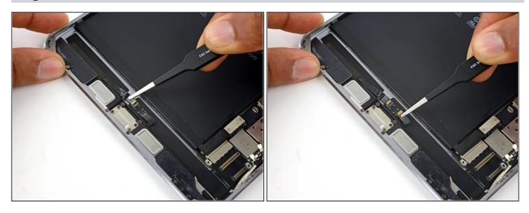
• Pull each speaker cable out from its ZIF socket.
