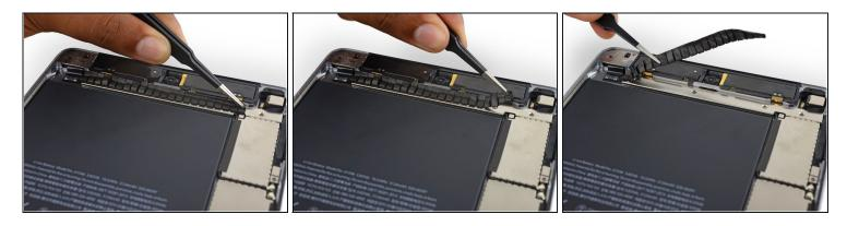
• Use <u>tweezers</u> to peel up the looped tape adhered over the upper component cable bracket.
