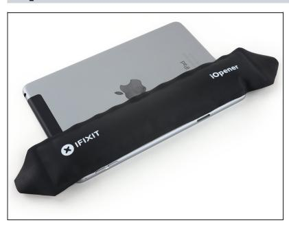
Reheat an iOpener and lay it on the backside of the iPad near the SIM slot for at least two minutes.
