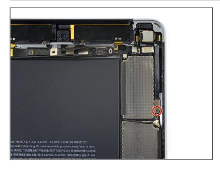
Remove the 1.2 mm Phillips screw securing the volume control cable.
