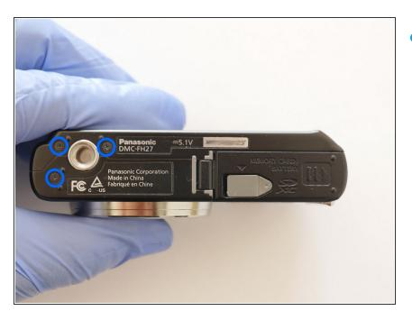
Remove 3 (0.4mm) screws from the base of the camera.
