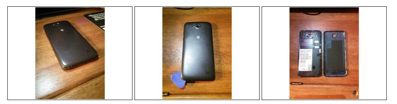
• Remove back cover using groove on bottom left corner of device.
