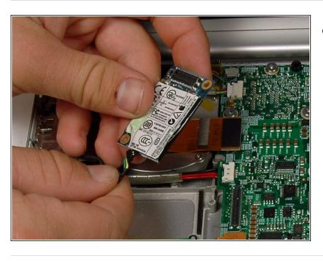
Disconnect the modem cable from the left side of the modem and remove it from the computer.
