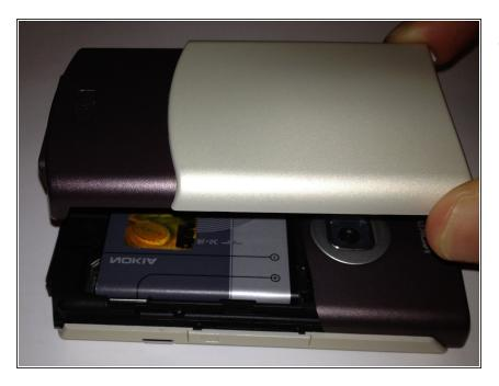
Remove the battery cover by lifting it away from the phone.
