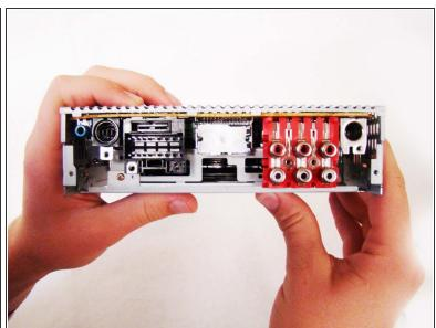
Firmly grip the body of the stereo and pull off the silver back plate.
