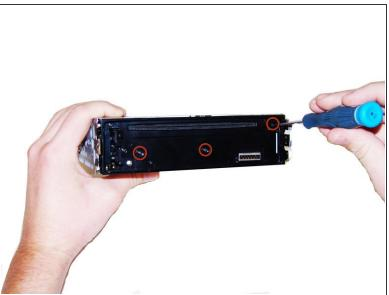
Using the <u>Phillips #0 Screwdriver</u>, unscrew the 3 screws (length - 7.5mm) on the front of the device.
