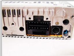
Carefully pull the fuse out of the back of the stereo.
