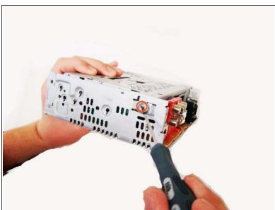
• Using the <u>Phillips #0 Screwdriver</u>, unscrew the 2 gold screws (length - 7.34mm) found on both sides of the stereo.
