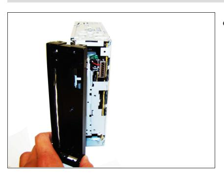
Remove the black front plate of the stereo.
