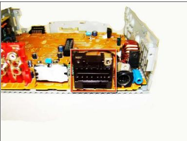
Remove the power supply on the circuit board. Please follow the <u>iFixit soldering guide</u> to assist you.
