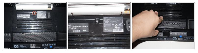
Unscrew the RAM door using a Phillips #1 screwdriver. Snap the RAM door off from the bottom and slide it off.
