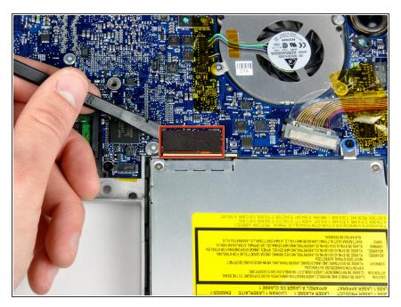
Use the flat end of a spudger to disconnect the orange SuperDrive ribbon cable from the logic board, removing tape as necessary.
