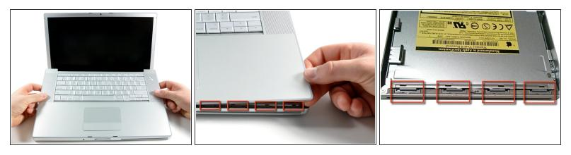
(i) Do not yank the upper case off quickly. The case is attached to the logic board via a ribbon cable.
