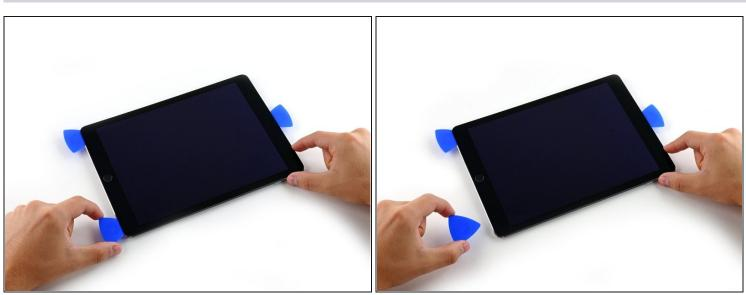
• Remove the right-hand opening pick at the bottom of the iPad.
