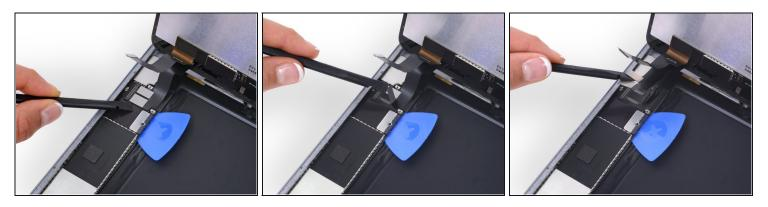
• Disconnect the two remaining digitizer cables underneath the display data cable.
