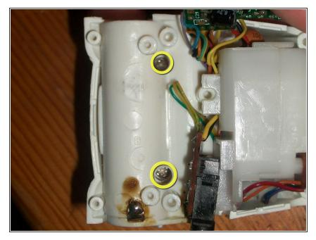
remove 2 screws accessed through battery housing. (Jack slides from motor housing and is easily resited it is not secured in place)
