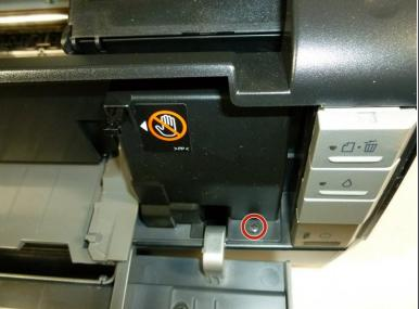
Remove the two 10 mm Phillips #2 screws on the front of the printer.
