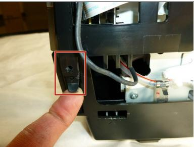
Detach the tabs from the pins on each side by pulling it outwards.
