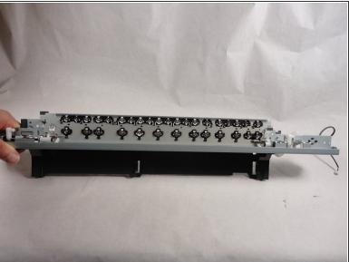
Remove the paper eject frame assembly by pulling it towards you.
