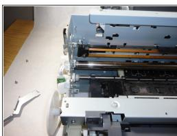
Detach the left frame support plate. Start by removing the two 6 mm screws that secure it and then pull it out by hand.
