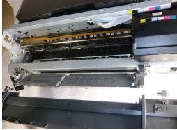
Remove the CD-R unit housing. Release the two attaching points to the tray base and then pull out the unit diagonally one side at a time.
