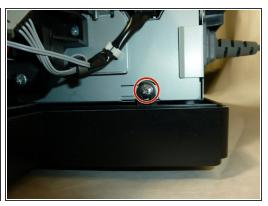
Remove the other three 10 mm screws that secure the printer mechanism using a Phillips #2 screwdriver.
