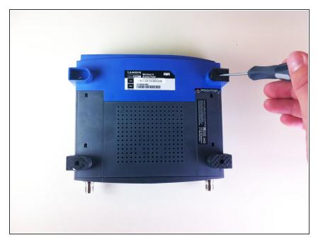
Remove the two black rubber feet of the device using the screwdriver. The feet are located on the bottom towards the front.
