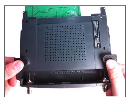
Now slide the bottom panel forward and remove it so the top casing is isolated from the bottom casing and motherboard.
