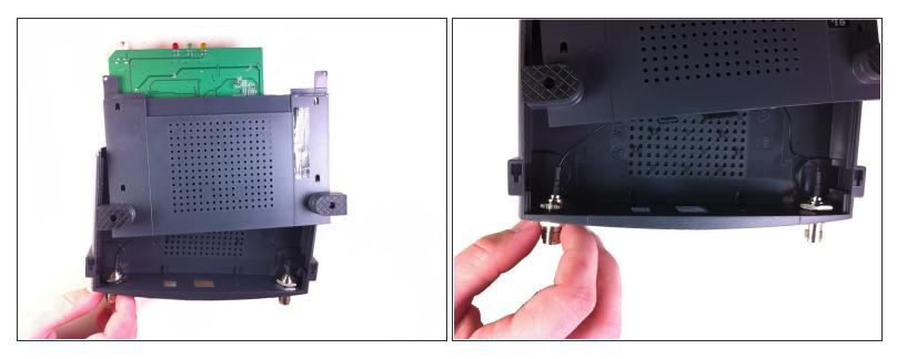
Unscrew the nut on the outer side of the back casing. Remove the nut and the washer from both antenna mounts.
