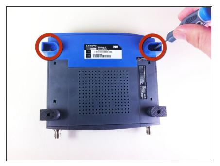
Once the feet are removed, two small screws will be visible. With a small screwdriver, unscrew them.
