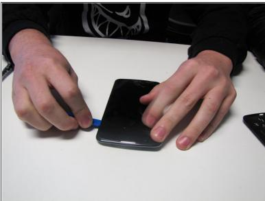
Unscrew all of the mid-frame screws, and use opening picks or a plastic opener to carefully remove the frame.
