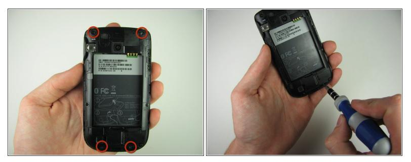
• Remove the four 4.9mm T6 Torx screws that secure the back panel to the rest of the phone.
