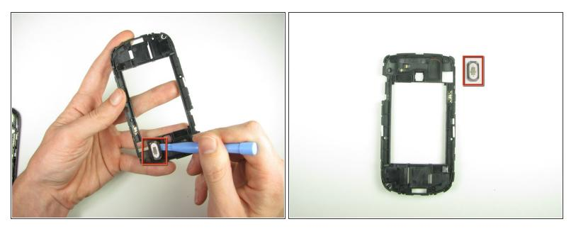
• Using the plastic opening tool, pry the external speaker out of the back panel.
