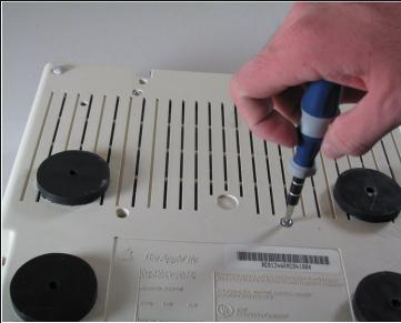
Carefully place device upside down to remove the four centered 21.1 mm screws that secure the floppy drive.
