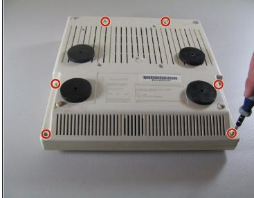
Remove the six 19 mm long screws with a #2 Phillips head screwdriver.
