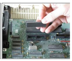
• Use the plastic opening tools to carefully lever the IC chips out of the holder. Gently lever one end and then the other to lift it out of the chip holder.
