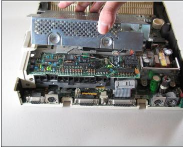
• Carefully lift the floppy drive cage straight up to remove it.
