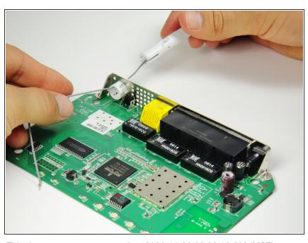
Pull out the antenna as well as the connected wire.
