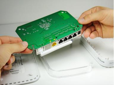
Separate the motherboard from the top shell by lifting it straight up from the router.
