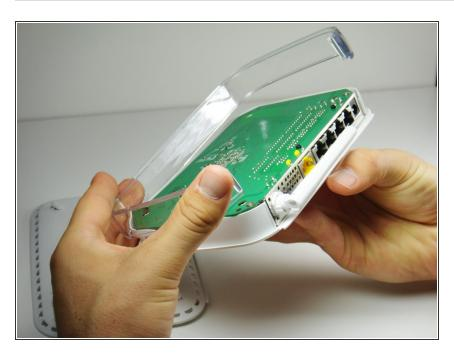
Remove the clear plastic casing by lifting it straight up from the router.
