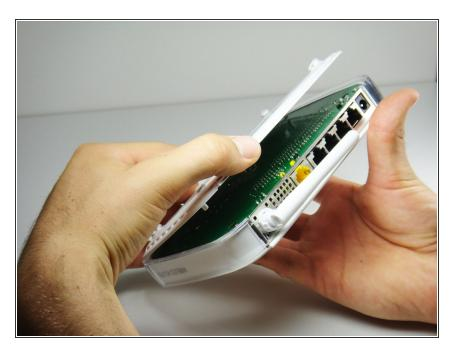
Lift the bottom casing straight up from the router.
