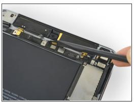
Use the flat end of a spudger to disconnect the front camera press connector from its socket on the logic board.
