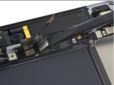
Use the flat end of a spudger to lift the headphone jack cable connector from its socket on the logic board.
