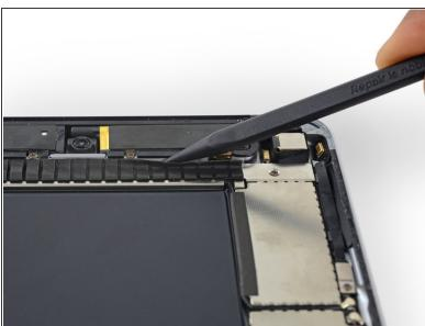
Run the pointed end of a spudger between the looped tape and the plastic cellular antenna housing to make it easier to peel the tape up.
