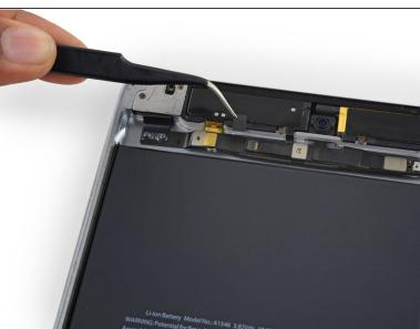
Use tweezers to remove the small piece of tape covering the the left antenna ribbon cable ZIF connector.
