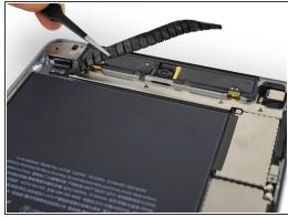
Use tweezers to peel up the looped tape adhered over the upper component cable bracket.
