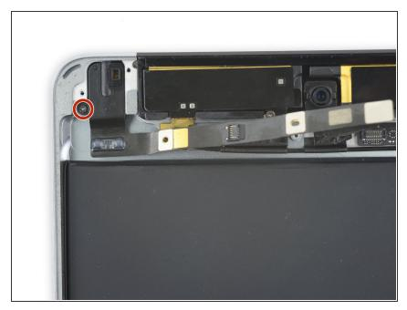
Remove the final 2.6 mm Phillips screw securing the headphone jack to the rear case.
