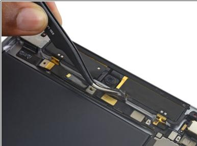
Peel up the tape over the front camera ribbon cable.
