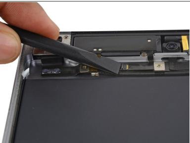
Use the flat end of a spudger to flip up the retaining flap on the left antenna ribbon cable ZIF connector.
