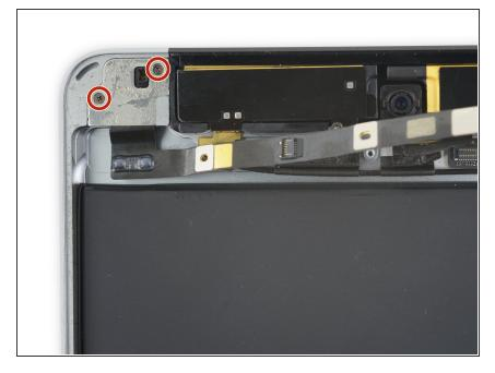
Remove the two 1.5 mm Phillips screws securing the headphone jack bracket.
