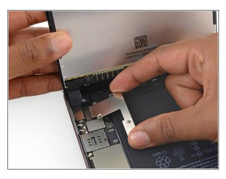
Remove the battery/display cable bracket.
