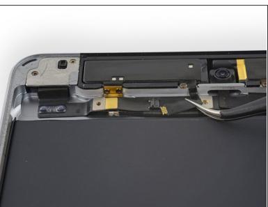
Use tweezers to pull the antenna ribbon cable from its ZIF socket on the headphone jack ribbon cable.
