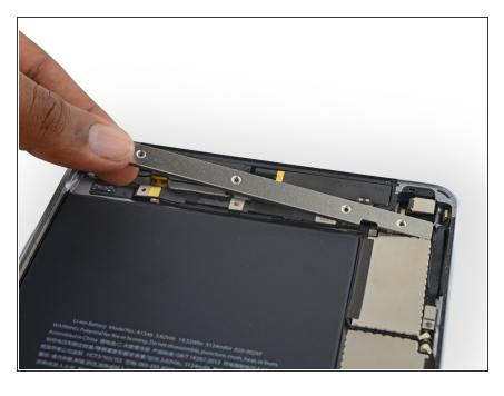
Remove the upper component cable bracket.
