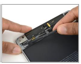
Slide the flat end of a spudger under the headphone jack ribbon cable to separate it from the adhesive holding it to the rear case.
