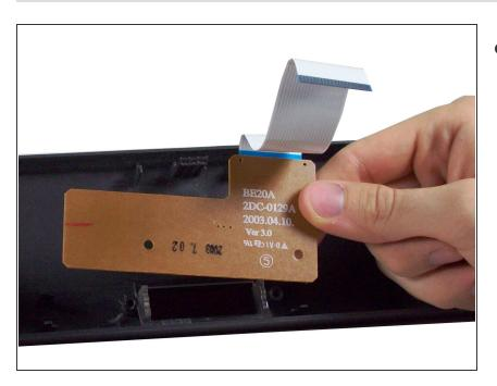
• Lift the sensor up to remove it.
