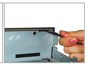
Use a spudger to push the three tabs on the inside of the front cover up and forward to release the cover.
