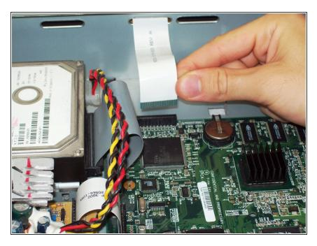
Unplug the ribbon cable from the motherboard. Some force may be required for this step, so be careful not to rip the ribbon cable.
