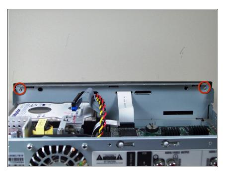
Unscrew the two 0.31 inch T-9 screws on the inside of the front cover.
