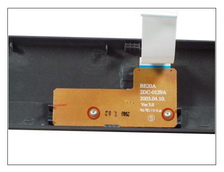
Unscrew the two 0.31 inch T-9 screws on the back of the sensor.
