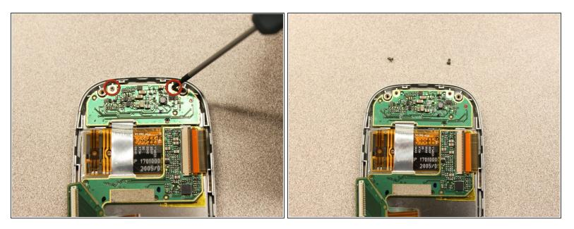
• Unscrew the two 3mm phillips #0 screws from the bottom of the device that secure the rigid flex board to the screen panel.
