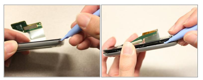
Insert the plastic opening tool between the front panel and the rear panel and pry open to reach the screen.
