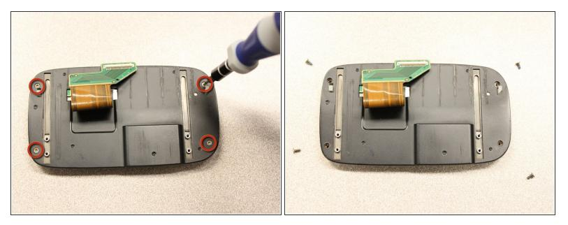
Use the T5 Torx screwdriver to remove four 5mm screws that secure the back of the screen casing.
