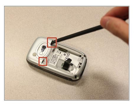
Insert the flat end of the <u>spudger</u> into the two notches on the back of the camera cover and pry them up.
