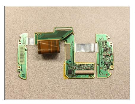
• Now that the rigid flex board is loose, remove it from the screen.
