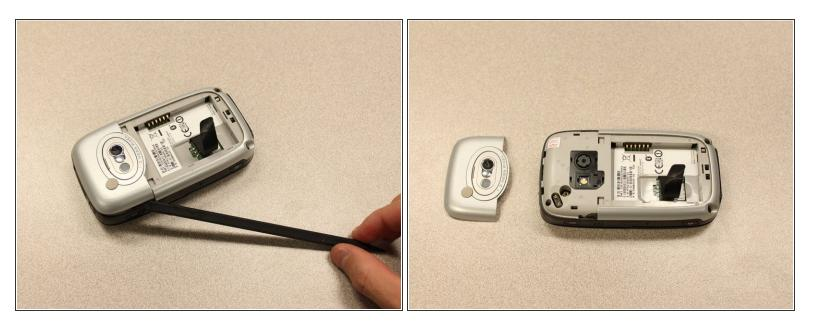
Work the <u>spudger</u> around the edges of the camera cover until it comes off.
