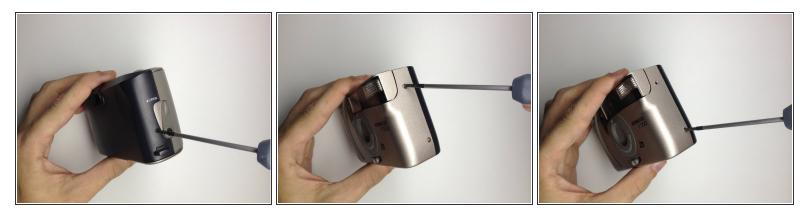
• Use the Phillips #00 Precision Screwdriver and remove the screws on the back cover.
