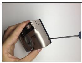
Use the Phillips #00 Precision Screwdriver and remove the screws on the back cover.
