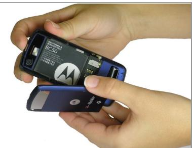
Press the panel release button on the top of the phone and simultaneously pull the rear panel away from the phone.
