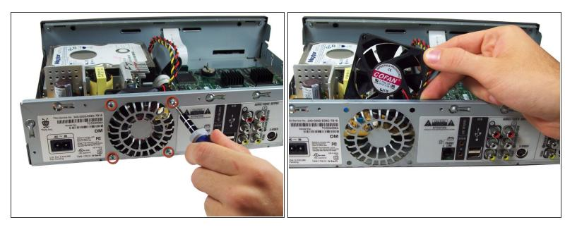
Remove the four 0.31 inch T-9 screws and gently pull fan out.
