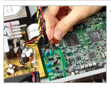
Remove power cable to fan from motherboard.
