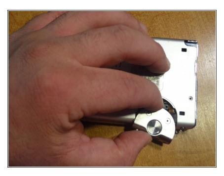
Remove the thumb dial panel by sliding it away from the device.
