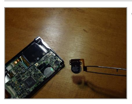
Pull plug straight up to remove from board.
