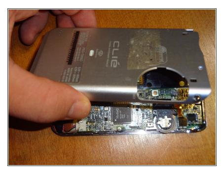
Remove the back panel exposing the inside of the device.
