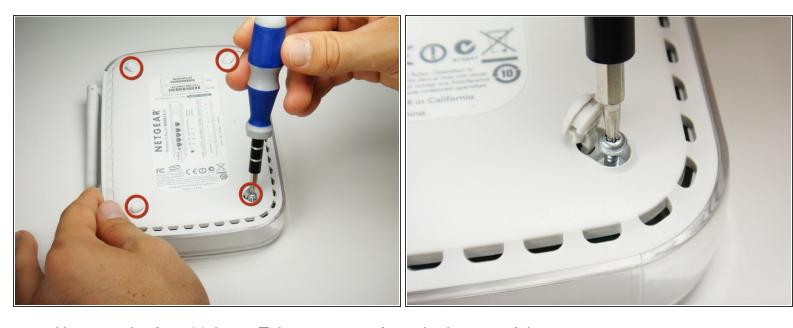
Unscrew the four 11.8 mm T-8 torx screws from the bottom of the router.
