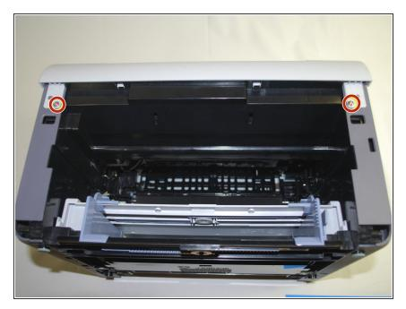
Using a Phillips #2 screwdriver, remove both 1" screws on the front face of the printer.
