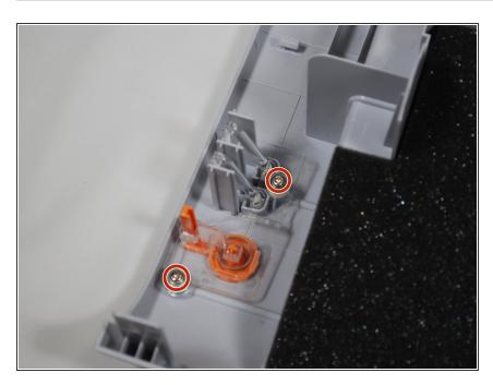
Using a Phillips #2 screwdriver, remove both 1" screws that secure the button to the underside of the top panel.
