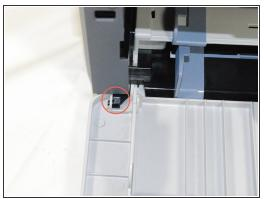
Remove the front panel by gently separating the holes on the panel from the pegs attached to the main printer body.
