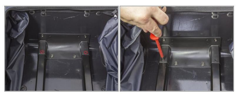
• Unscrew the two screws in the lower section on the handle assembly using a Phillips screwdriver.
