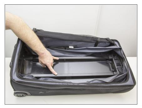
Open the zip inside the trolley to expose the handle.
