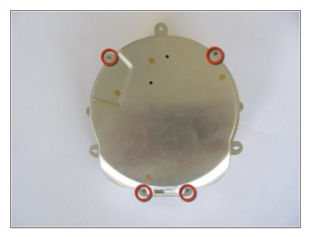
Remove four 1mm phillips screws from the bottom.
