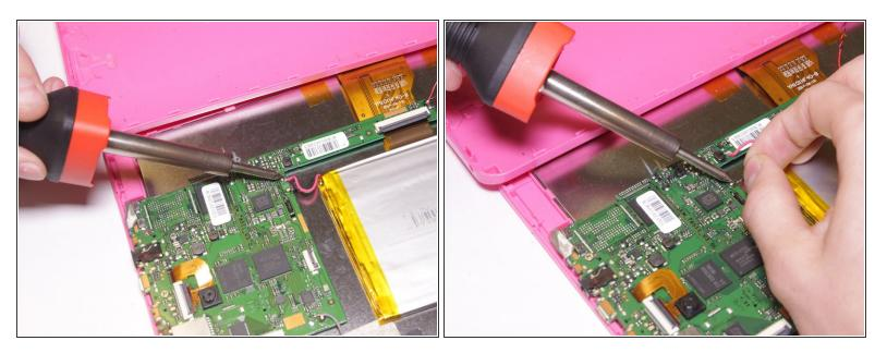
• Use a soldering iron to melt the solder then remove the red and black wire from the motherboard.
