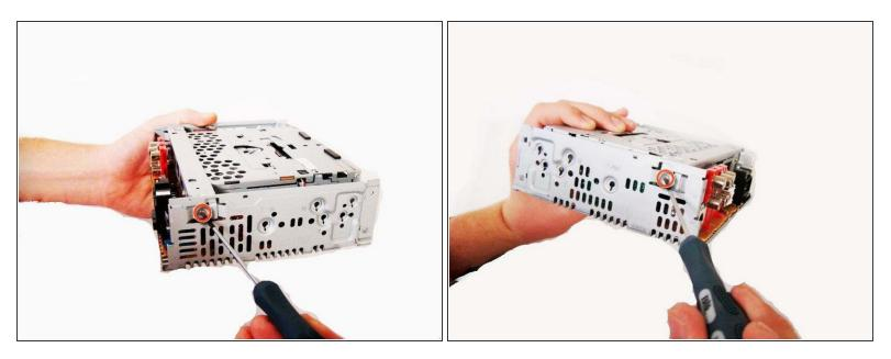
Using the <u>Phillips #0 Screwdriver</u>, unscrew the 2 gold screws (length - 7.34mm) found on both sides of the stereo.
