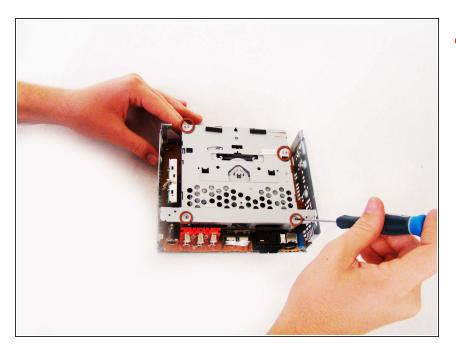
Using the <u>Phillips #0 Screwdriver</u>, unscrew the 4 dark-silver screws (length - 3.71mm).
