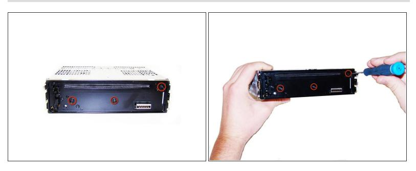
Using the <u>Phillips #0 Screwdriver</u>, unscrew the 3 screws (length - 7.5mm) on the front of the device.
