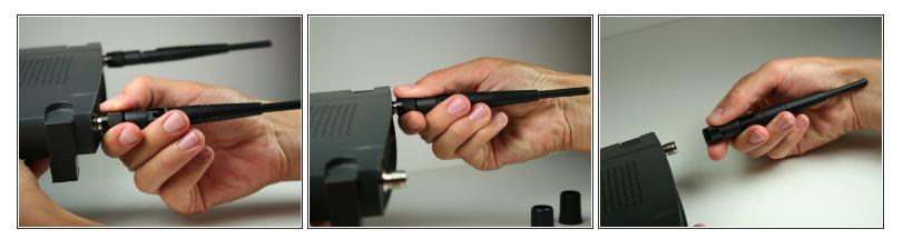
• Unscrew each of the antennas from the wireless device.
