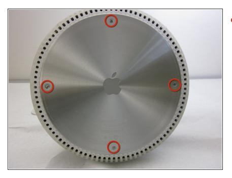
Loosen the four Phillips #0 screws.
