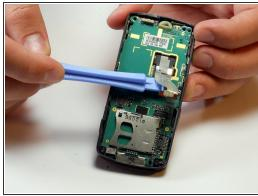
Using a plastic opening device, push against the underside of the brown portion of the the ribbon cable to unplug it.
