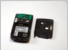
Run a plastic opening tool along the edge of the back casing while prying it apart to remove it.
