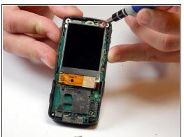
Remove the indicated 6.35mm screws with a Torx T6 screwdriver.
