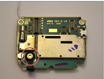
Replace the entire motherboard to replace the microphone.
