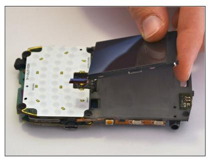
With your fingers, carefully remove the screen so as not to damage it.
