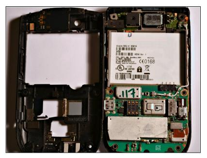
Using the <u>iFixit Opening Tool</u> or your fingers, remove the midframe of the phone.
