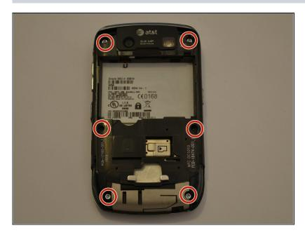
Using a <u>T6 Torx screwdriver</u>, remove the six screws.
