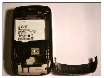
Using the iFixit <u>Opening Tool</u>, remove the lower rear cover.
