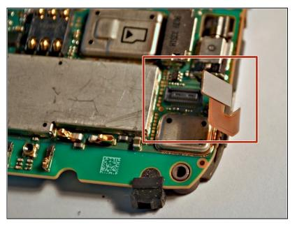
Detach the ribbon cable on the front of the motherboard using the <u>Spudger tool</u>.
