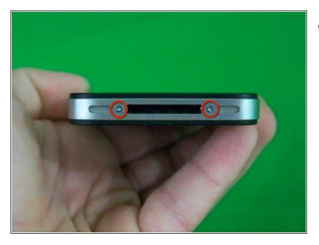
Using a 5-point pentalobe screwdriver, unscrew the 2 pentalobe on the bottom of the phone near the dock connector.
