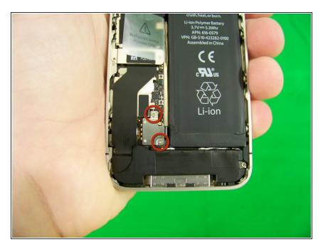
Using a #000 Phillips screwdriver, unscrew the 2 very small Phillips screws.
