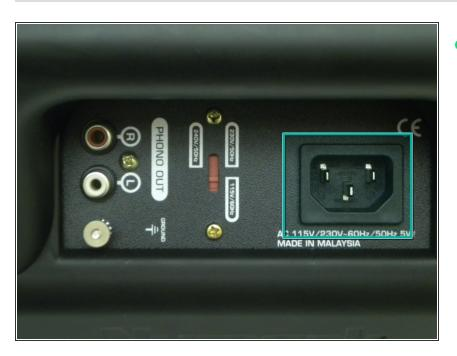
Insert power cable into socket.
