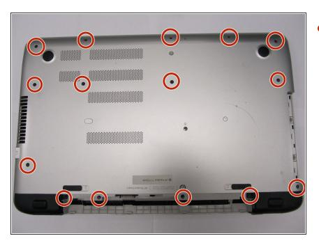
Remove fifteen 7 mm screws with a Phillips #1 screwdriver.
