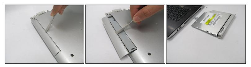
• Use a metal spudger to push the CD drive out of its slot for removal.
