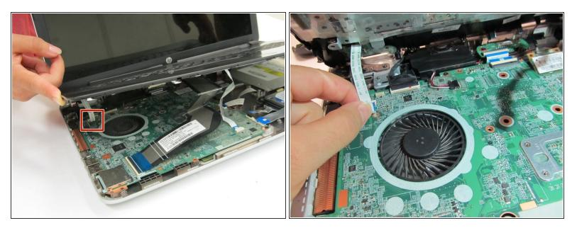
Remove the ribbon connecting the power button to the motherboard.
