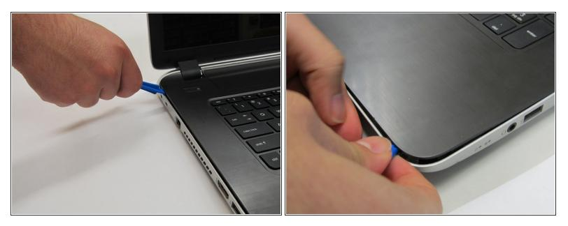
• Flip the laptop back over. Then, with the laptop open, move the plastic prying tool around the top cover to pry it from the enclosure.
