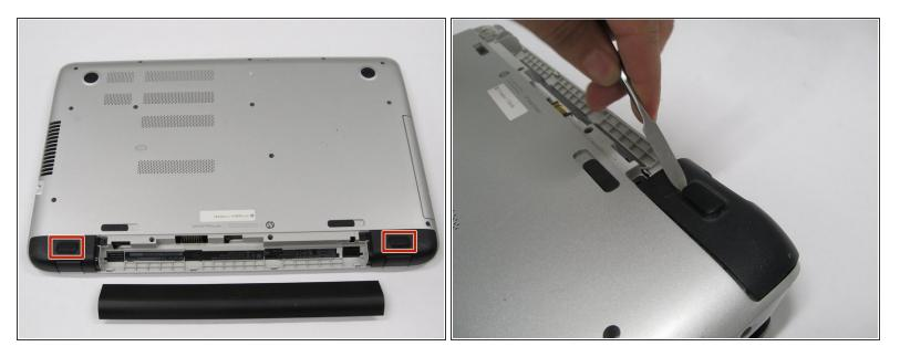
• Use a metal spudger to remove the rubber "feet" to expose two screws.
