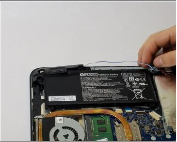
• Use the nylon spudger to pry away the blue/white wire that is positioned near your battery.
