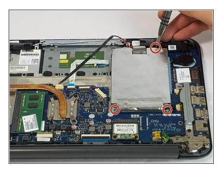
Use the Phillips #0 to remove the three 3mm screws holding the hard drive in place.
