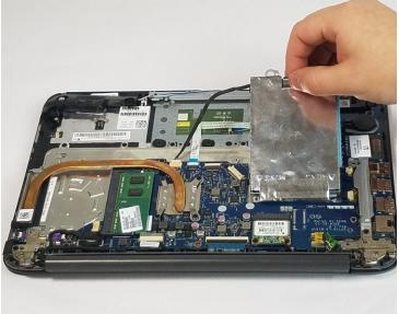
• Carefully lift the hard drive out of place using the tag.
