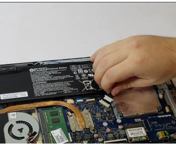
Disconnect the battery cable from the motherboard by carefully pulling on the black wire at the point closest to the white tab.
