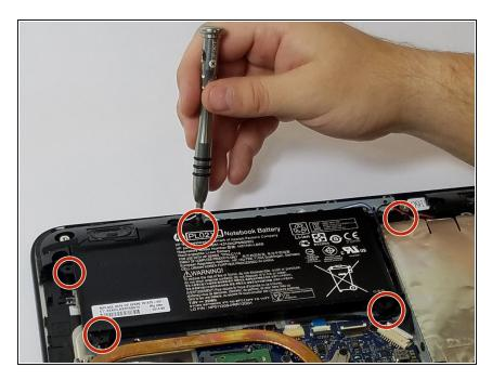
Remove the five 6mm screws that hold the battery in place using the Phillips #0.
