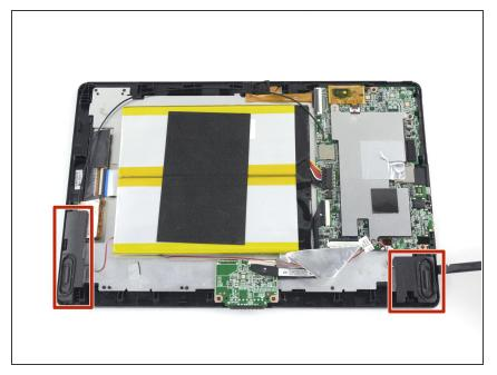
Use a spudger to lift the speakers out of the device.
