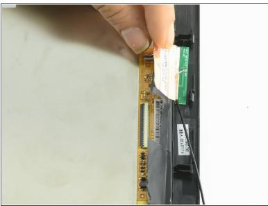
Peel the protective flap away from the display.
