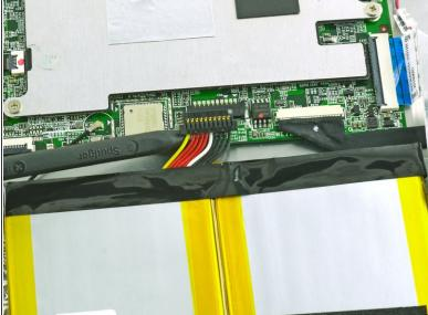
Use a spudger to disconnect the black bundled cable connector from the motherboard.
