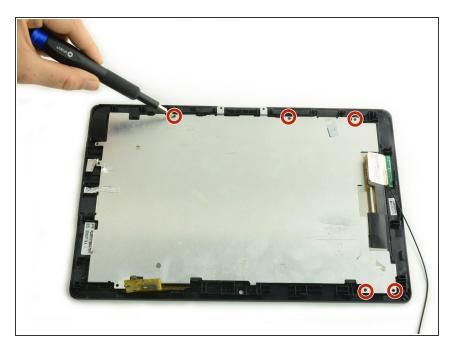
Unscrew the five 4.2mm screws with a Phillips #000 screwdriver.
