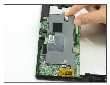
Lift the protective shield away from the motherboard.
