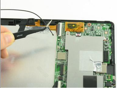
• Use ESD safe tweezers to disconnect the antenna from the motherboard.
