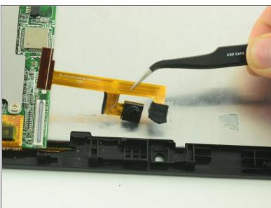
Use tweezers to lift the camera assembly away from the device.
