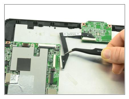
Use tweezers to pull the dock connection cable away from the motherboard.
