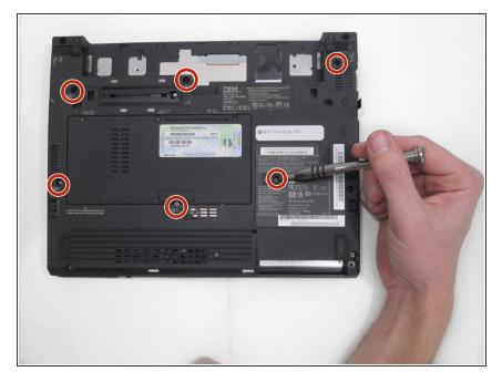
With a Phillips PH000 to remove all six 6 mm screws identified for the keyboard as shown.
