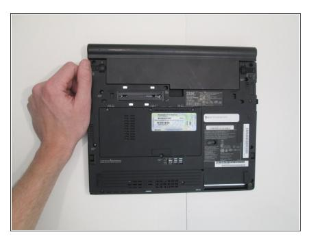
Locate battery release button lock on laptop, and press down.
