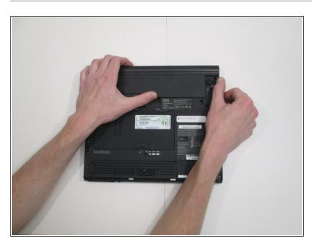
Hold laptop battery release button and gently pull battery away from laptop.
