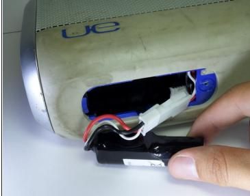
• Expose the battery by gently pulling it away from the battery cavity.
