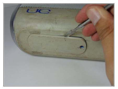
Pry off the rubber battery cover using a metal spudger.
