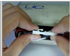
• Firmly press down on the end of the latch and pull connector apart.
