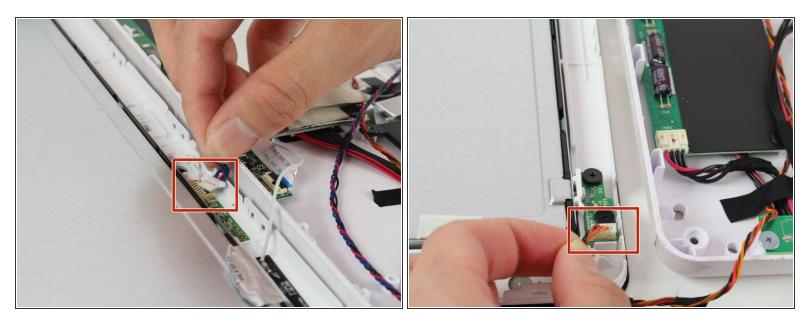
Carefully grab both sides of the white plastic piece with your fingers and gently pull directly upward.
