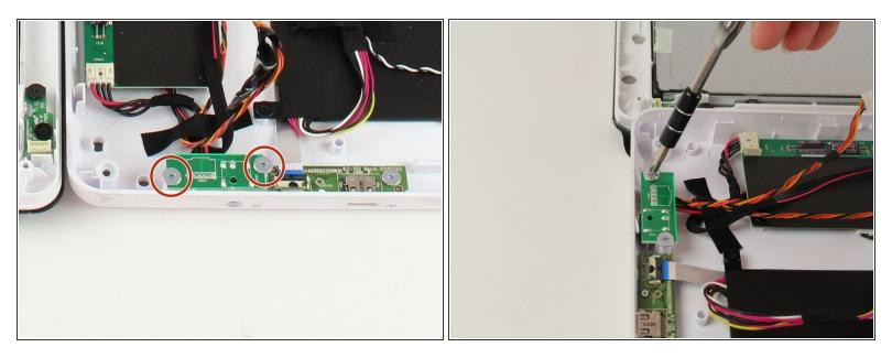
Use a Philips #1 screw driver to unscrew the two silver 4.5 mm screws located on top of the circuit board.
