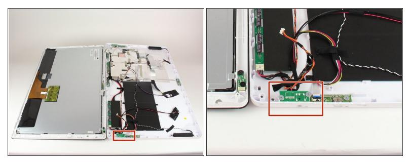
Locate the battery charging port labeled "DC" on the side of the tablet .
