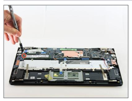
Remove the one 2mm Phillips #1 screw holding the hard drive to the laptop.
