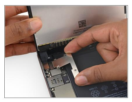
• Remove the battery/display cable bracket.
