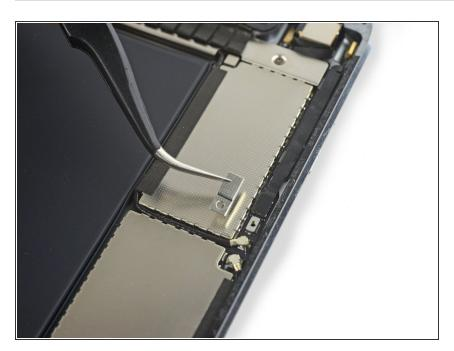
• Remove the volume control cable bracket.
