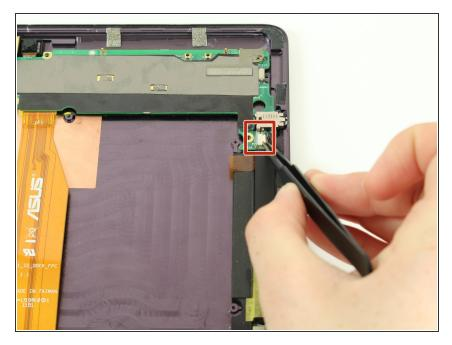
Disconnect the speaker assembly from the motherboard by using precision tweezers to unplug the white plug from its tan receptacle.
