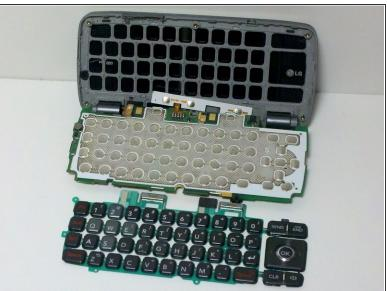
Pull the rubber keyboard off carefully.
