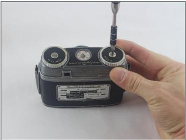
• Using the <u>2.5mm flathead</u> screwdriver, remove both 2.8mm flathead screws that hold the wind and rewind dials in place. Then, remove the washer located underneath each dial.
